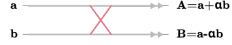
Figure 5: Diagram of butterfly operations for complex multiplication and addition. This diagram clearly indicates the source of data for each output.
